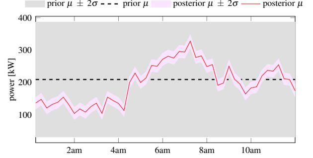
Figure 4: Example of priors calculated using (1) and posteriors using (2) for predicting power consumption of a building for 12 hrs. Initially the mean is constant because  $\mu(x)$  is constant, and we observe a high variance. The posterior agrees with the actual power consumption with high confidence.
