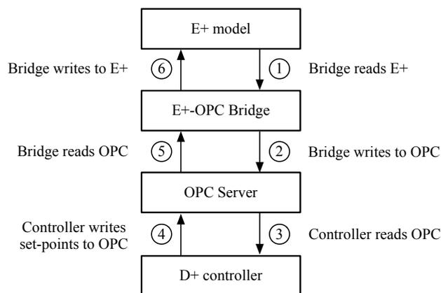
Figure 3: Communication sequence for data exchange.
