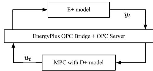
Figure 2: The MPC controller runs in Python using the D+ models and applies the optimal inputs to the E+ model. The communication is made possible using the `pyEp` library and the OPC connection.
