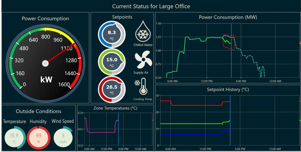
Figure 6: Status of the LargeOffice as seen on SCADA system during Demand Tracking Control. The blue vertical line shows the current time of operation. Power consumption: the baseline power consumption is shown in dashed line, the curtailment is shown in solid green and the 95% confidence bounds are shown in solid red. Since a fixed curtailment is tracked without thermal comfort constraints in problem (4), the zone temperature shoots up by 2°C.
