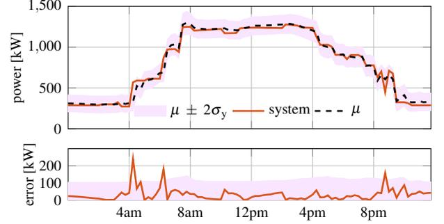
Figure 5: Rolling forecast of the power demand for one particular day using GP model  $\mathcal{M}_1$ . The actual demand is almost always within the 95% confidence interval.
