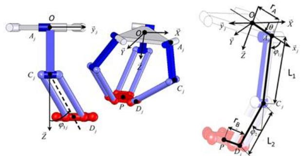
Figure 3 Geometry of Delta Robot [3]
