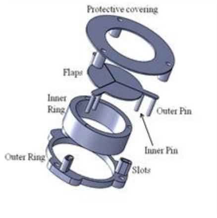
Figure 4: Exploded view of end effector
