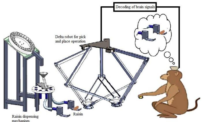
Figure 10: Teleoperation through BMI: A schematic
