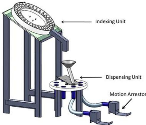
Figure 8: Raisin Dispensing Mechanism
