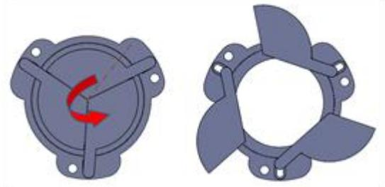
Figure 5: Anti-clockwise rotation of inner ring opens the shutter (right)
