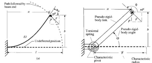
Figure 6: Deflection in cantilever beam and (b) Approximation of this bending by rotation about a pseudo joint
