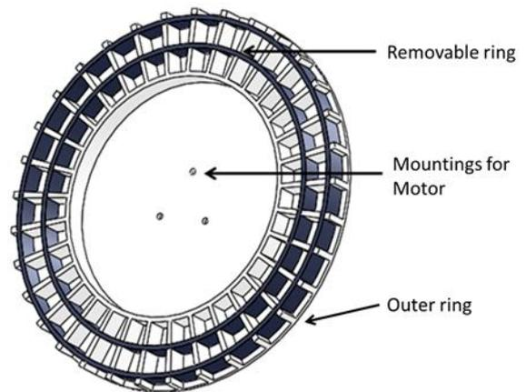
Figure 9: Indexing disc
