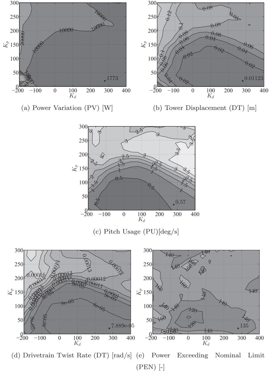
Fig. 5. Performance of a conventional PID controller in Region 3 as a function of  $K_p$  and  $K_d$  for  $K_i = 1$ .
