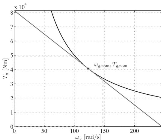
Fig. 6. Linearized power constraint with region of feasibility.
